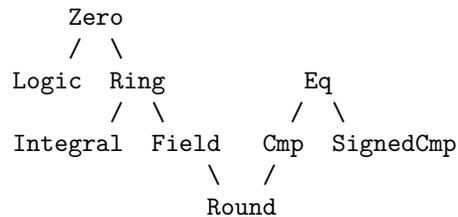
This diagram describes how the various typeclasses in Cryptol are related. A type which is an instance of a subclass is also always a member of all of its superclasses. For example, any type which is a member of `Field` is also a member of `Ring` and `Zero`.
